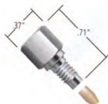
UP-F-140 10-32 Stainless Steel Nut with F-142 PEEK™ Ferrule
